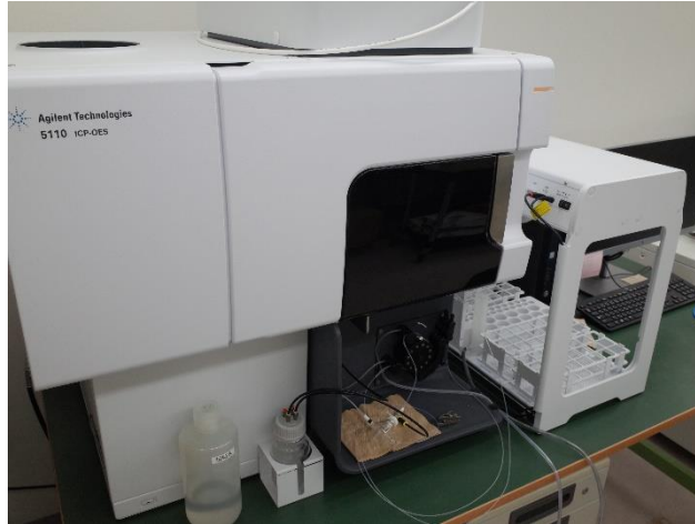
ICP Luminescent Spectrophotometer (elemental analysis such as sodium)
