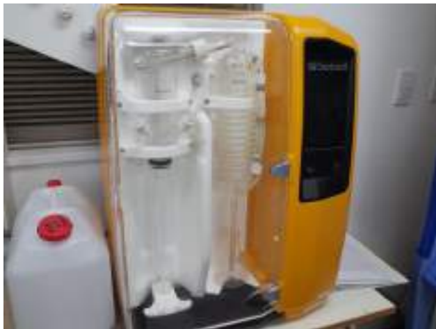
Kjeldahl distillation Device (for protein)
