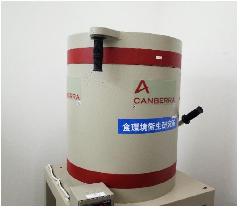
Germanium-based Semiconductor Detector (for radiation test)
