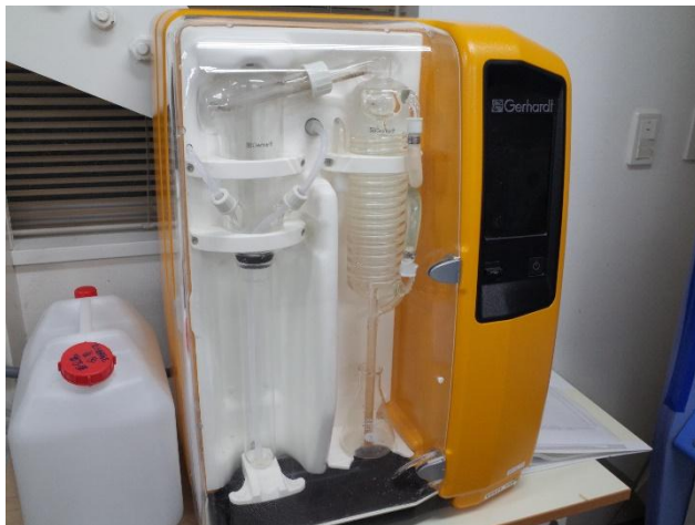
Kjeldahl distillation Device (for protein)
