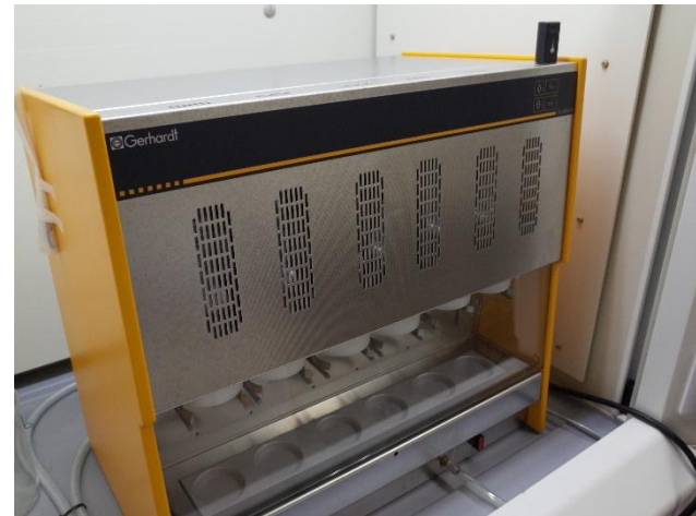
Fully automated Soxhlet Device (for lipids)
